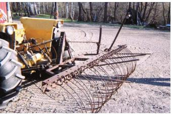
Gabe Davidson removed the wheels and seat from an old horse-drawn rake, then made brackets to mount it on a tractor 3-pt.
