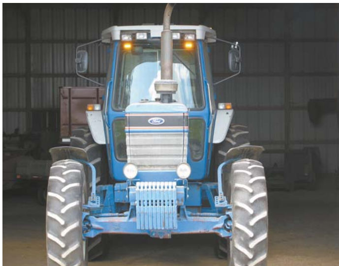
Tim Mack converted the factory-supplied incandescent warning lights on his tractor to mini, high intensity LED lights.
