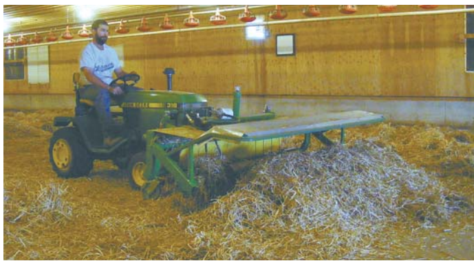
Rotary fork mounts on the push blades of most small utility tractors, making it easy to spread straw in poultry barns.
