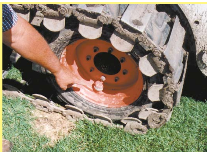
To keep valve stems from snapping off on his skid loader, Cassidy welded a threaded gas pipe nipple over them.
