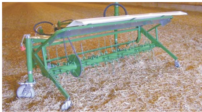
It takes Campbell an hour to spread straw in a 25,000 sq. ft. building with his rotary fork.
