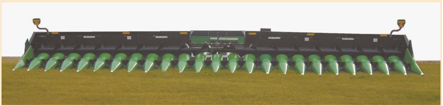
Clarke Machine's 24-row, 20-in. spacing header features a double drive system, in which the four inside rows on each side are driven separately off a gearbox. The other eight rows on each side are shaft-driven off both ends of the header.
