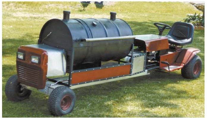
John Benoit extended the frame on a 1989 Montgomery Ward riding mower to 11 ft., converting it into a self-propelled grill.
