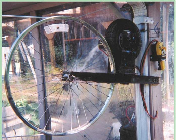
A 12-volt winch motor is bolted to a 10-in. rubber drive tire, which is positioned so it rubs against the metal bike wheel.
