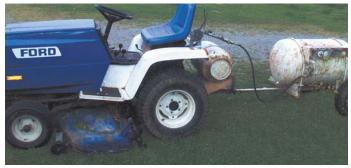
Richard Turner's Ford lawn tractor is equipped with a standard Kohler 10 hp gas engine that can be powered by either gas or natural gas.
