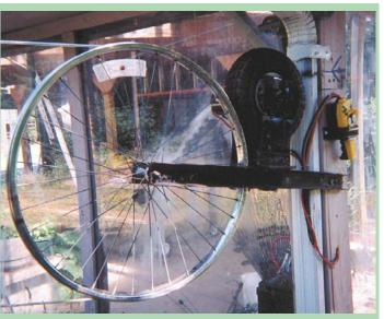
A 12-volt winch motor is bolted to a 10-in. rubber drive tire, which is positioned so it rubs against the metal bike wheel.
