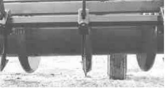
Hydraulically-adjustable shank openers ahead of each wheel help maintain consistent furrow depth and also plow rocks out of the way.
