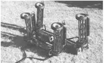
Mower's steel frame allows the two rows of reels to flex forward and backward, and each reel can flex up and down to prevent scalping.
