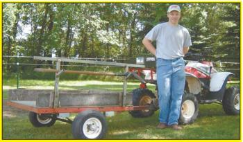
I made a tool rack out of chrome-plated square tubing. The rack has two pieces of square tubing cut at a 45 degree angle and they stick out to hold the tool. The rack mounts to a 2-wheeled, 4-ft. long commercial trailer with four bolts. It works great when I fill up dog and
