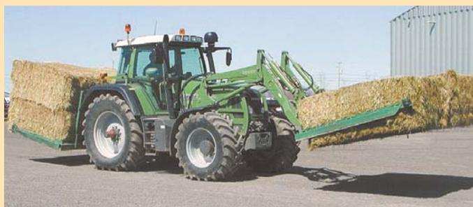
Depending on the model and the tractor/loader combination, an operator can pick up one to six bales at a time.
