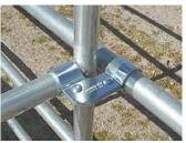
Clamp is used to connect two corral panels by attaching the horizontal rail of one panel to the horizontal rail of the second.
