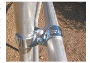
Pole clamp has a figure-8 twist that allows the connection of vertical and horizontal pipes.
