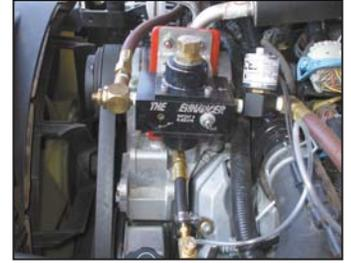
for particulate emissions," relates Ridgeway. "With our propane valve installed, his truck dropped from 11 percent particulates to zero."
