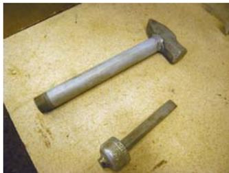
A chisel is welded to a metal end cap that screws onto one end of pipe, with a hammer head welded to the other end.
