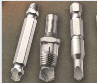
3/8-in. bolt. “Drill-out” is a broken bolt extractor, consisting of a drill-bit and extractor in one tool. “X-out” is designed to remove damaged screws by simply applying pressure on the fastener head with a reversible power tool. Or, it can be used manually with a ratcheting screwdriver.
