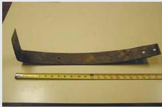
ends since it already had pretty thin ends but some springs would probably need that. The bar works great for removing wood trim without scarring, and the curved section is useful for lifting sheet rock an inch or so into position. I’m sure there will be many other uses I haven’t thought of yet.”
