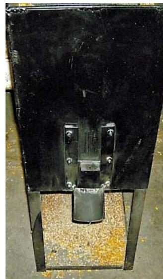
Corn bounces off the sloped screen, through a sliding door, and into a 5-gal. bucket.
