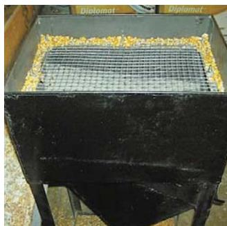
Top of corn cleaner box has a screen selected for its kernel size. The sloped bottom is also a screen.
