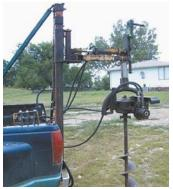
Egli's pickup-mounted, hydraulic-powered post auger (left) and post driver.
