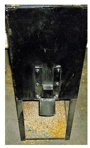
Corn bounces off the sloped screen, through a sliding door, and into a 5-gal. bucket.
