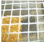
Top of corn cleaner box has a screen selected for its kernel size. The sloped bottom is
