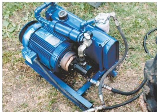
Motor shaft drives a 2-stage hydraulic pump, with a lovejoy coupling used to couple the pump to the motor.
