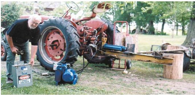
John Youngdahl put together this tractor-mounted splitter out of scavenged parts. "It's powered by an electric motor so it's quiet and produces no exhaust fumes," he says.
