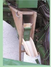
Lightweight wooden chute is designed to set under planter's seed tank.
