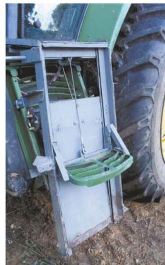
Battery-operated winch raises and lowers step on homemade metal slide.
