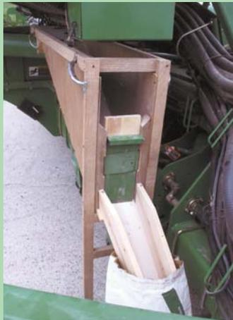
Lightweight wooden chute is designed to set under planter's seed tank.
