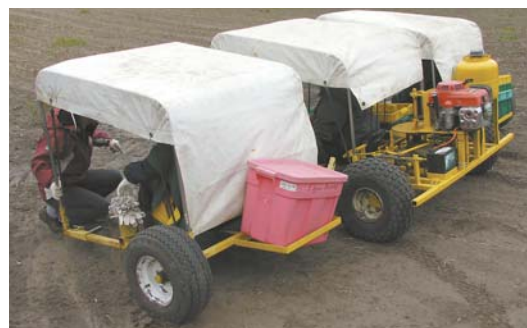
Foot steering makes it easy for pickers to lean forward and pick asparagus between their legs.
