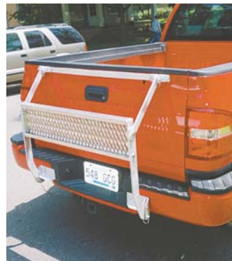
Add-on step bolts onto pickup's bumper and also onto back side of tailgate.
