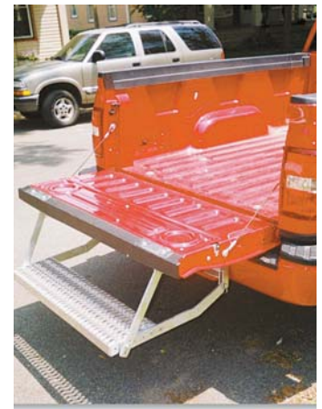
Add-on step bolts onto pickup's bumper and also onto back side of tailgate.
