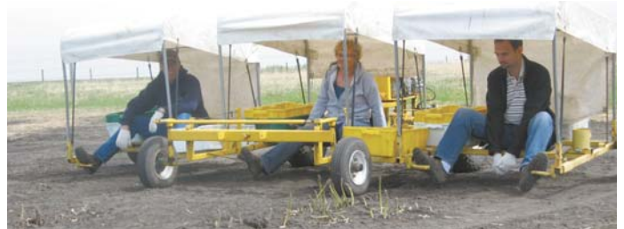
Foot steering makes it easy for pickers to lean forward and pick asparagus between their legs.
