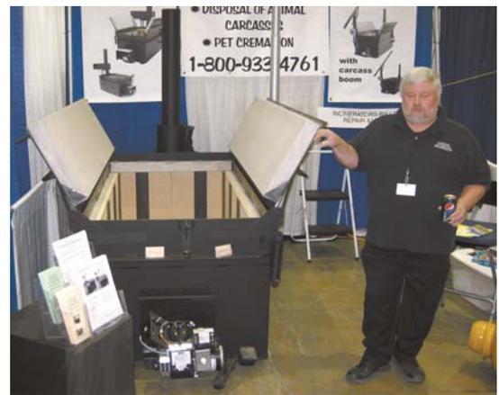
to two scoop shovels of ashes in a few hours. He estimates that once in operation, the incinerator can dispose of up to 150 lbs. of dead animals per hour.
