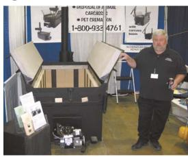
to two scoop shovels of ashes in a few hours. He estimates that once in operation, the incinerator can dispose of up to 150 lbs. of dead animals per hour. Contact: FARM SHOW Followup, Larry Lewis Livestock Incinerator, 3045 Snyder Ave., Cedar, Iowa 52543 (ph 641 933-4762 or 800 933-4761).
