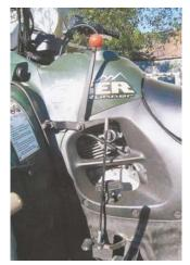
Shifter fabricated out of 3/8-in. rod connects to ATV's foot pedal.
