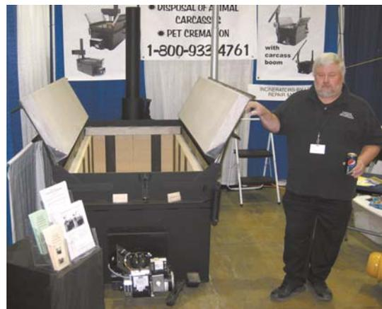
to two scoop shovels of ashes in a few hours. He estimates that once in operation, the incinerator can dispose of up to 150 lbs. of dead animals per hour.
