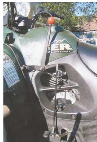
Shifter fabricated out of 3/8-in. rod connects to ATV's foot pedal.
