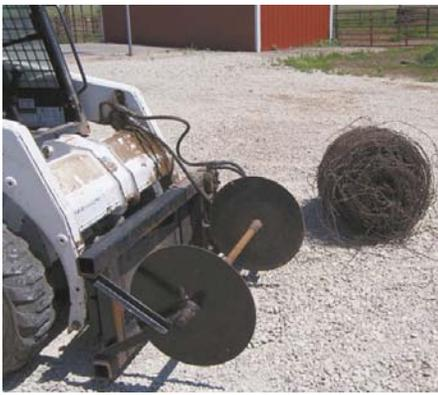
Home-built wire roller can roll up 1/4 mile of fence in only about 10 minutes.
