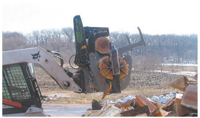
System lets operator pick up whole logs, saw them to firewood lengths and split the blocks, all without leaving the skid steer seat.
