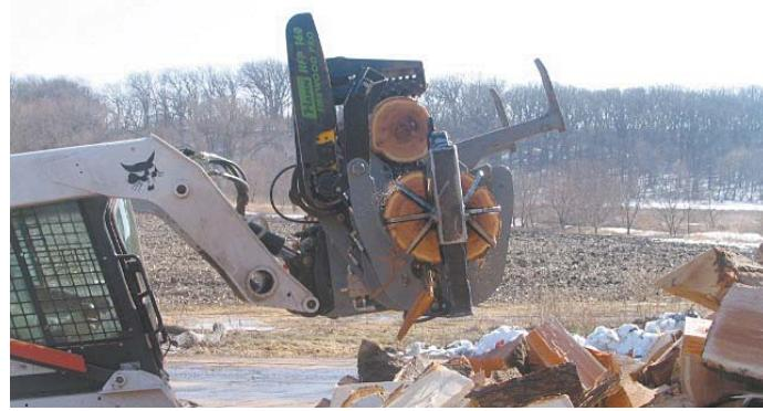
System lets operator pick up whole logs, saw them to firewood lengths and split the blocks, all without leaving the skid steer seat.
