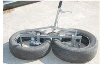
Machine shoves a screw through two tires, quickly fastening them together.
