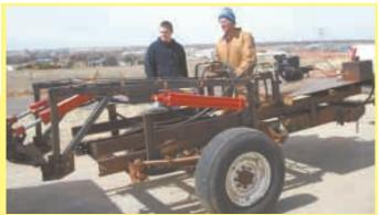
Big bale mover is built on an old pickup bed. "It lets me retrieve bales stacked two high on a trailer and stack them in my barn, without needing a tractor," says Windle Tucker.
