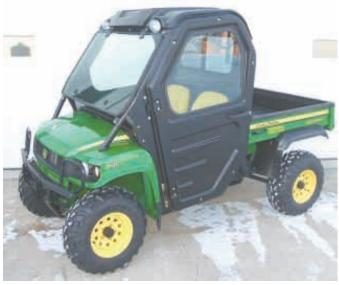
Cab bolts onto Gator's standard rollover protective structure. Cab's roof and doors are made from heavy-duty ABS plastic and mount on a steel frame.
