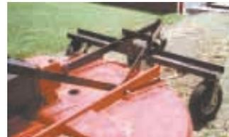
He U-clamped a 6-ft. length of channel iron onto the frame horizontally behind deck, then bolted a caster wheel onto each end. ground on uneven terrain. I got the idea from commercial mowers I've seen that use a similar system," notes Donk.
