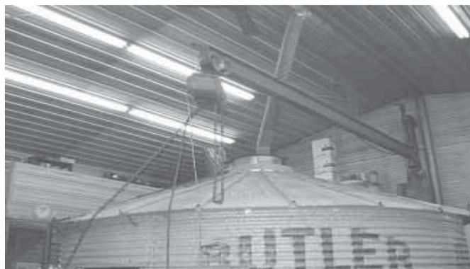
Once the bin is inside his shop, Gutschmidt attaches a section of ventilation hose to an adapter he added to top hatch of bin. A fan pulls dust and paint fumes out of building.
