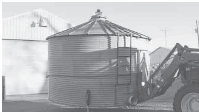
Roger Gutschmidt turned a 1,000-bu. steel grain bin into a portable sandblasting and paint booth. He uses a front-end loader to move it in or out of his shop as needed.
