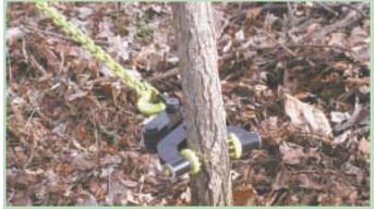
A pair of 360 degree-rotating "grip pads" attach to spring-loaded, scissors-type jaws that tightly grip tree trunk when pulled backward.
