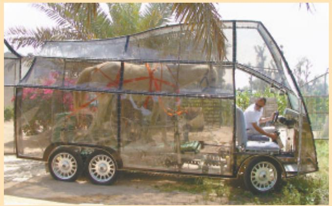
Horse walks on a conveyor belt, which activates a 36-gear transmission to move vehicle forward. A transparent plastic body lets spectators watch it work.
