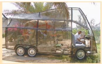
Horse walks on a conveyor belt, which activates a 36-gear transmission to move vehicle forward. A transparent plastic body lets spectators watch it work.
