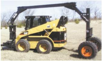
Cattail towbar system is designed to accept a wide variety of tools and attachments.
