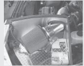
Intake on a 7.3-liter Powerstroke diesel.
