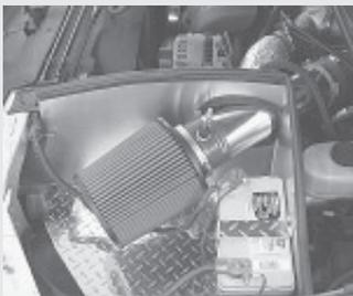
**Intake on a 7.3-liter Powerstroke diesel.**
