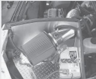
**Intake on a 7.3-liter Powerstroke diesel.**
