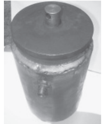
Filter housing heats veggie oil before it enters engine by plumbing into the engine coolant lines.
