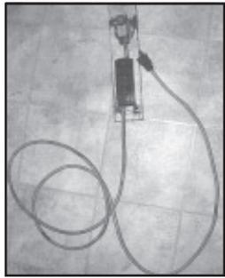
one end of a small flat metal plate and the limit switch to the other end and then wired them together. The extension cord plugs into any wall outlet.
