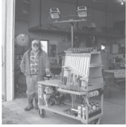
light can be pulled out from a retractable reel, and there's a strip of electrical outlets where you can plug in power tools.
