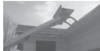
Lee Dietsch built this lightweight elevator, attaching a pair of metal feet to lift elevator above roof edge and rain gutters.
