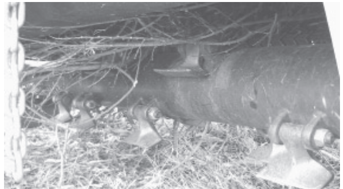
Heavy flail knives on front turn on a 2,200-rpm motor.
