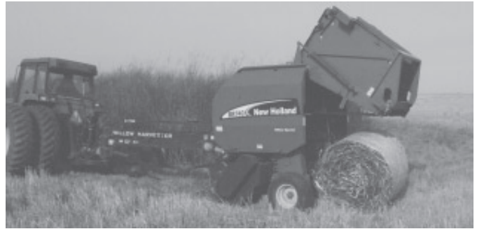
Standing trees up to 4 in. in diameter are compacted into round bales that handle like conventional round bales.
