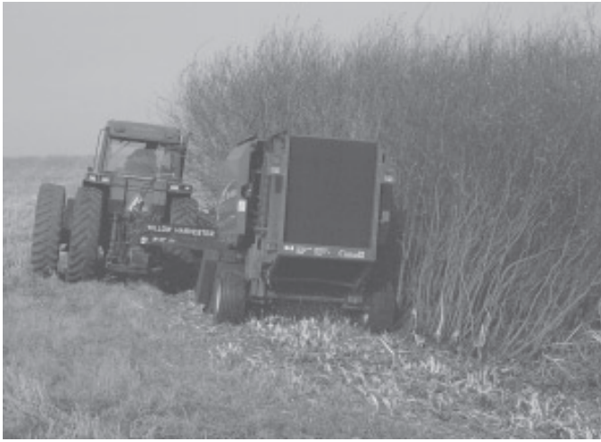
Biobaler has flail knives on front that cut young trees, feeding them into bale chamber.
