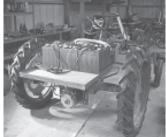
Electric motor and sprocket assembly attaches to clutch plate and clutch housing/transmission (left). Battery power storage mounts on frame above motor.
