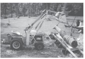
Chain attached to bucket hooks onto either end of log.
