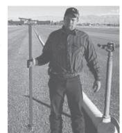
Ryan Sweat says his new "Riserench" saves time and water when repairing broken risers in wheel line irrigation systems.
