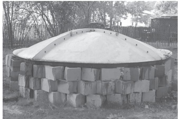
Satellite dish is turned upside down on three rows of concrete blocks, with the blocks in each row set at different angles for better ventilation.
