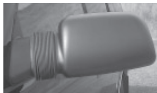
Extending mirror is electrically-operated, extending with the flip of a switch.
