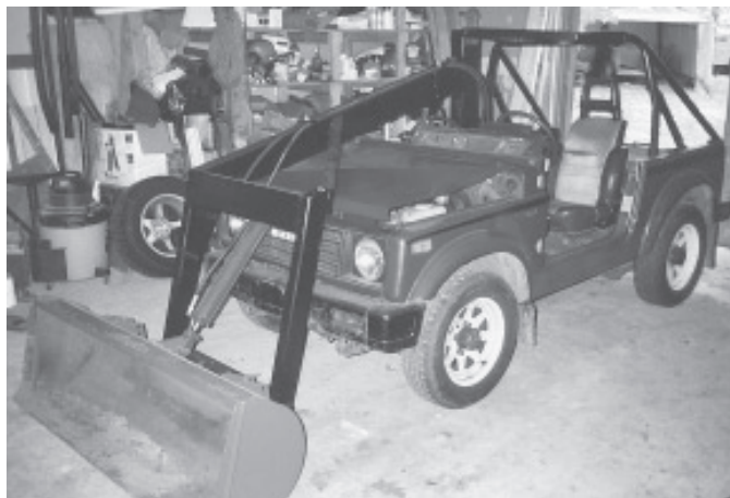
Jeff Weeks built a frame to attach a 5-ft. bucket to his Suzuki. One-post mounting provides a great view from the driver's seat.
