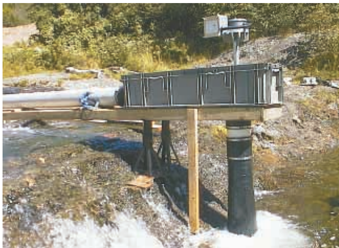
Stream Engine produces 300 watts of continuous power, enough to run a house with lights, well pump, refrigerator and other appliances.
