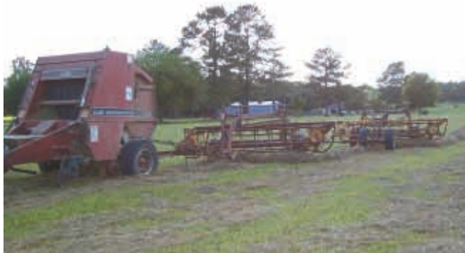
Hitch attaches to baler axle, allowing Burks to tow two right-side delivery rakes behind baler. They swing behind baler for road travel.
