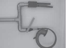
Air-powered doorbell combines the sound of an antique car horn and a homemade train whistle.
