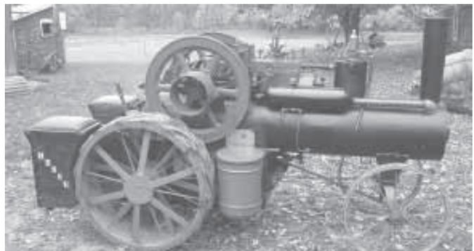
Boiler is a 16-in. piece of natural gas pipe, with power supplied by a 6 hp engine.
