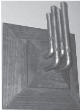
A whistle built for a friend consists of four pieces of 1/2-in. dia. copper pipe with notches in them, and plugs in the ends to restrict the air.
