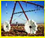
have a tractor tire lug design that fills up with mud, causing the wheel to spin and get stuck. The cleats on our wheel are deep and are spaced farther apart. Also, they go straight across both sides of the wheel like the lugs found on old-time tractors with steel wheels. The result is that they're far less likely to get stuck.
