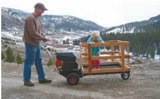
Moulton's 3-wheeled, self-propelled cart is powered by a 4 hp engine. The single caster wheel on front is located about 4 ft. ahead of the rear wheels.
