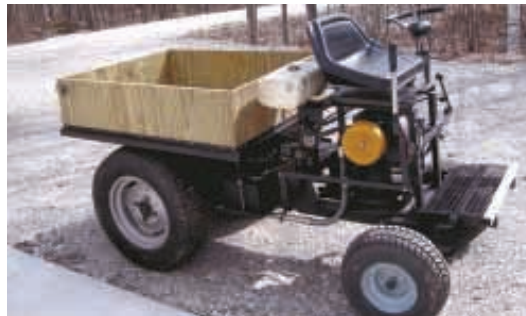
"Gator wannabe" is built on an old White garden tractor. The driver's seat and controls were moved forward over the motor and front end.
