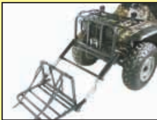
Telescopic arms retract to lock load into position for transport.
