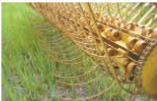
Specially-built tines revolve slightly slower than machine's forward movement.
